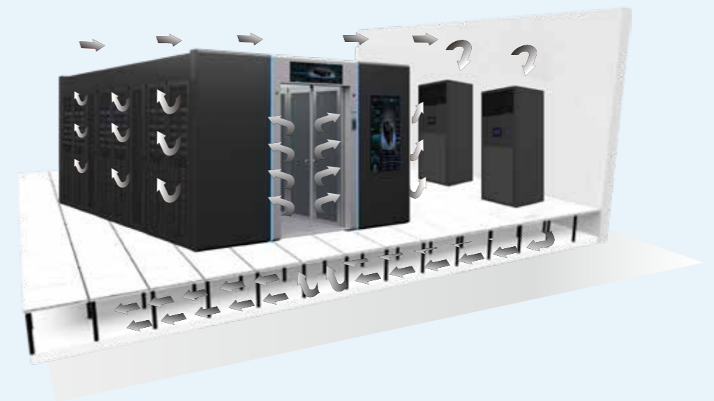
Room-level Cooling Airflow
